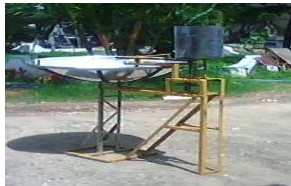
Figure 2: Experimental Setup of the Pyroelectric Energy Harvesting System
