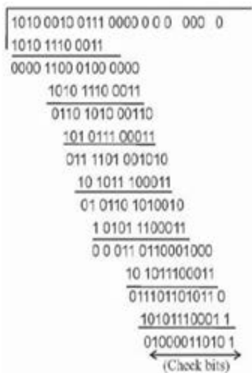
Example of check bits generation.
