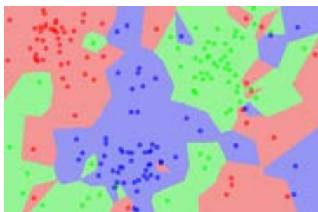
Fig. 3 shows the 1NN classification map: each pixel is classified by 1NN using all the data
